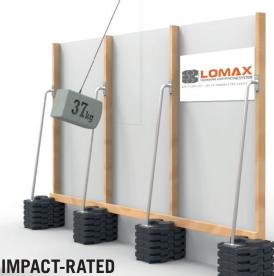
Pre-certified and impact tested from both the front and rear of the hoarding for compliance to AS4687
